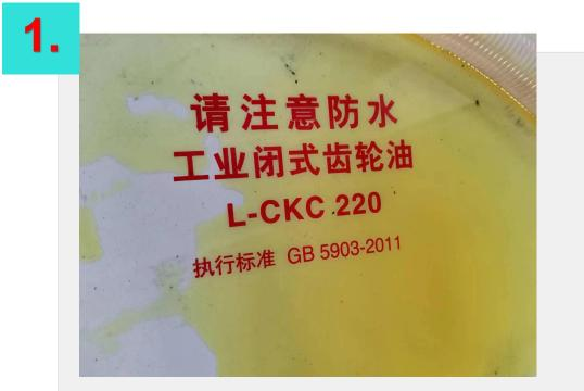
减速箱齿轮油 Gear oil for reduction gearbox
